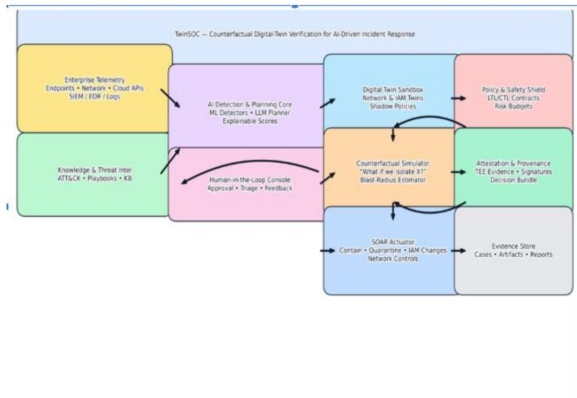
**Figure 1:** TwinSOC architecture showing the flow from telemetry and intelligence into AI detection and planning, counterfactual verification inside a digital twin, policy-safe decisioning with attestations, and controlled execution through the orchestration layer.
